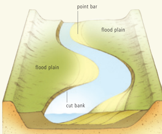
Anatomy of a Meandering Bayou. The water current is constantly eroding the outer bend, which creates a cut bank, and carrying sediment and depositing it further downstream on the next inside bend, which creates a point bar.
